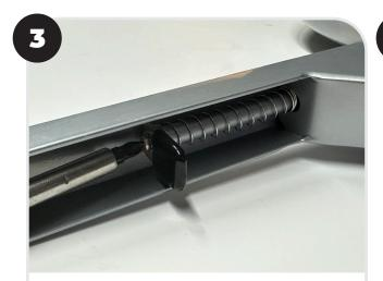
Place the spring over the metal rod. Hold the tab on the end of the metal rod. Tighten the small screw into the end of the rod as tightly as possible (this is where inserting something rigid in the hole at the previous stage helps).
